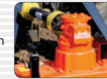
Single speed gear box for 540 RPM PTO
